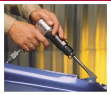
Ingersoll-Rand air hammers are designed so you can let the tool do the work, whether it's cutting, punching, chipping, or scraping. Each air hammer comes with a coil spring retainer for fast and easy chisel changes. You can also get the Ingersoll-Rand air hammer kit, which includes the five piece chisel kit, or buy them separately.
