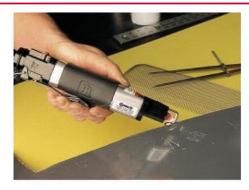
The Ingersoll-Rand air shear, air nibbler, and air reciprocating saw give you speed and power plus tight accuracy for intricate shapes and details. For example, the IR4429 reciprocating saw features increased durability and a composite handle surface for greater comfort and control. It also includes an easy-to-use exhaust hose attachment for a cleaner working environment.
