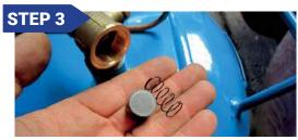
Check the face of the seal making sure that there are no foreign objects present, or that the wear depression is not excessive. Wiping the face of the seal on a rag can remove any objects from the seal.
