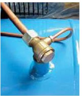
The Non Return Valve (NRV) has a very important role in the operation of the compressor. Its primary function is to stop the back pressure in the air receiver tank being forced back into the compressor pump.
